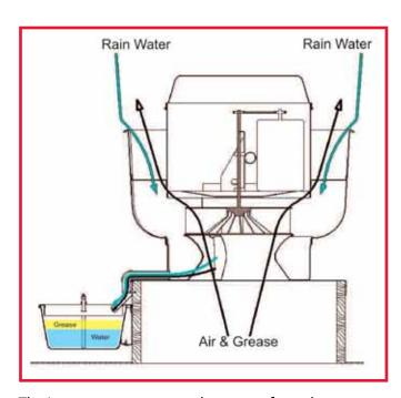
The Interceptor separates the grease from the water. The liquid grease remains in the Interceptor and clean water flows freely out of the unit.
